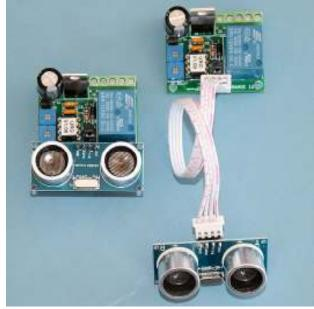
Connections on J1 from left to right: +V GND NC COM NO
