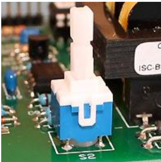
Use flat washer for spacer under switch.
