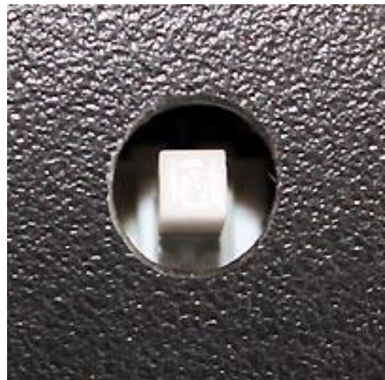
Carefully center switches in cover holes.
