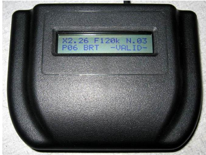
The XTBM displays X10 signal voltage, carrier frequency, and last decoded X10 command. It also displays powerline noise, and will indicate various types of errors that plague X10 communication, including the ubiquitous “bad start code”. The average frequency of sufficiently strong “in band” noise is also displayed.
