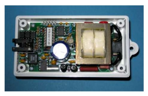
Many of you are familiar with the XTB and XTB-IIR X10 Transmit Boosters that have been available since 2006. Like the other XTB units, the XTB-XM outputs a much stronger signal than normal X10 transmitters. It can deliver over 20Vpp onto the powerline. When combined with a good tuned-circuit passive coupler like the XPCP, the XTB-XM located near the distribution panel can provide strong signals throughout an average home.
