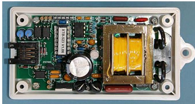
Borrowing from the XTB-IIR, the XTB-523 goes way beyond the basic functionality of the simple TW523. Its transmitter is based on the XTB design, and produces a much stronger signal than other X10 transmitters. Depending on line characteristics, the XTB-523 can deliver 20Vpp or more at 120KHz onto the AC line.
