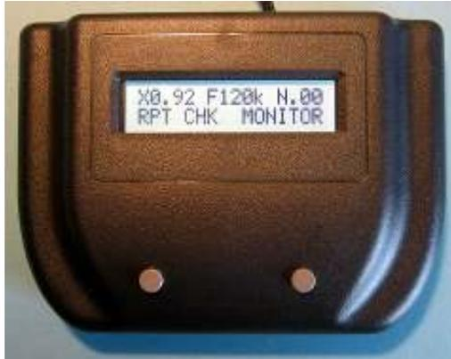
Both meters will display the peak-to-peak signal level of each decoded X10 command in the form Xx.xx (Vpp). Resolution is 10mV. Valid decoded commands are displayed, as are any errors that corrupt X10 communication.
