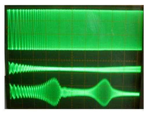
In this plot the frequency is swept linearly from 20KHz to 220KHz, with 120KHz (the X10 bandpass) at the center. The excitation scale factor was 2V per cm. The filter outputs were 200mV per cm. A resistor was inserted in series with each filter to prevent loading down the signal generator and causing interaction between the two filters. (Without the resistor, the peaks on the XPF are much larger as that series-resonant circuit sucks energy from the signal generator.)
