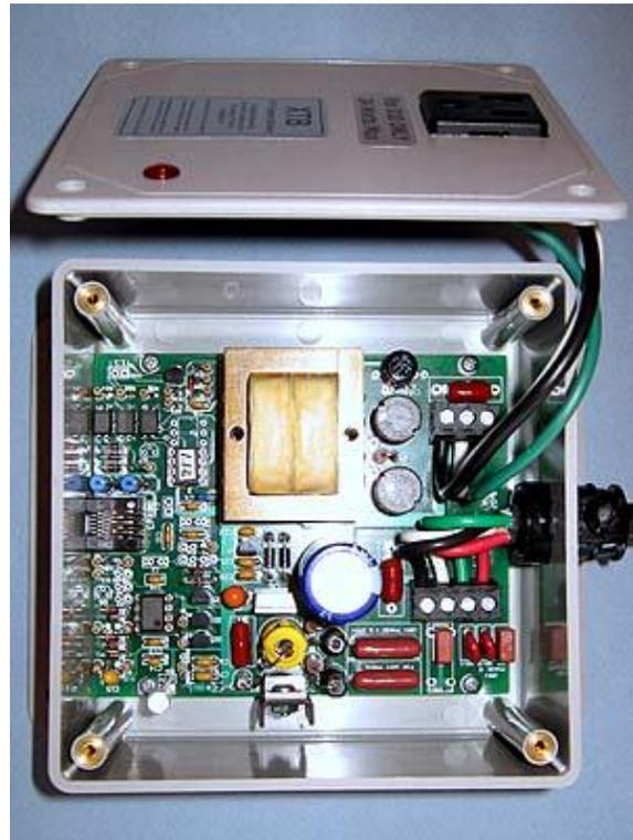
The original XTB Transmit Signal Booster    XTB-II 2-phase Transmit Signal Booster
