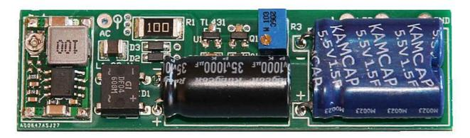
The LED Light Strip Voltage Regulator will maintain constant brightness of a 5V LED light strip installed in a model railroad passenger car. It uses a super capacitor to provide up to 10 seconds of constant power even if track power is interrupted for block control. It eliminates any blinking as cars traverse switches or have intermittent pick-up contact.
